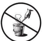
Use an 80 grit silicon carbide (or "green") wheel to sharpen carbide, or use diamond pads. Always air-cool carbide; never dip it in water or oil to cool it.
